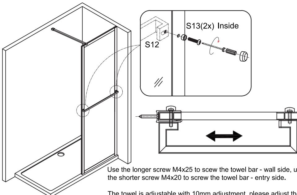
Use the longer screw M4x25 to screw the towel bar - wall side, use the shorter screw M4x20 to screw the towel bar - entry side.
