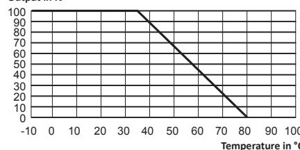
When in operation, the dimmer becomes warm as a small proportion of the connected load is transformed into heat. The nominal output of the dimmer, as indicated, is designed for installation in solid stone or concrete walls.
