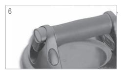
Remove the suction cup lifter from the suction surface. When the vulcanised rubber disc "sticks", raise the disc from the side with a finger so that air can get underneath. The "sticking" occurs occasionally with new discs of vulcanised rubber and does not adversely affect its functionality.
