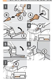
Work securely and carefully, follow the instructions. It is advisable to practice following the instructions by making a 'dry' run (without sanding disc, without rotary sanding roller) beforehand. You must feel confident of a correct and smooth operation beforehand! Before sanding, test the sanding results on an unobtrusive place and convince you of the correct result.
